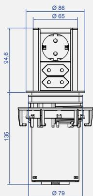
ELEVATOR fits in cut-outs 79 mm in diameter
